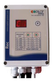
Regulator installed in the recovery system
